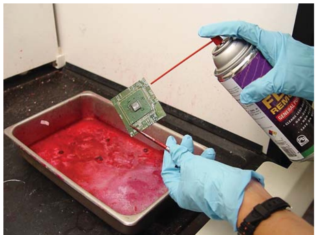
Figure 6 Sample Being Cleaned With Spray Flux Remover After Liquid Cleaning
