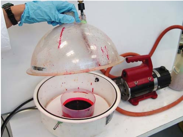
Figure 7 Dye Vacuum Station – Sample Completely Submerged in Dye
