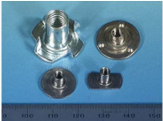
Figure 9 Sample Prepped With Tee Nut, Pull Hook and Molding Compound (Top) and Examples of Tee Nuts (Bottom)
